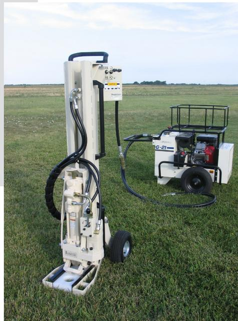
The 420M unit being powered by the PortaCo® hydraulic power unit. (Left). The 420M can also be powered off of other hydraulic sources including larger Geoprobe Systems® machines with auxiliary hydraulics.
