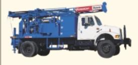
The B-59 driveline is the heart of this rig's exceptional performance. The fully-reversing Clark power shift transmission is equipped with 3 speeds forward and reverse. Combined with our field-proven 2-speed right angle drive, the B-59
